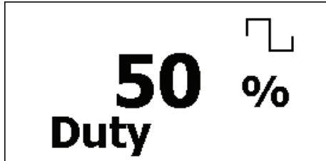
When setting Square wave output, pressing the **DUTY⑪** key will enter duty cycle adjustment mode. Press number key to set duty cycle percentage, ranges between 20~80%. After setting the value, press **Enter②** to execute duty cycle adjustment.
